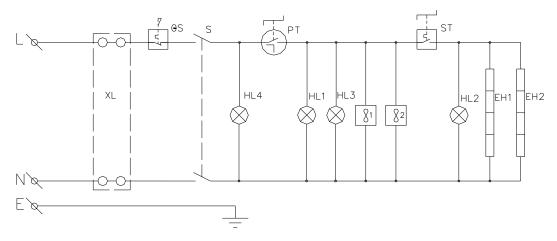
XL--- Wire Connecting Terminal $\theta$  S--- Temperature LimiterS--- Operating SwitchPT---TimerST--- ThermostatHL1/HL2---TimerIndicatorHL3/HL4---Interior light/Heating lamp $\infty 1. \infty 2$ --- Draught FanEH1.EH2--- Electric HeatingElement
