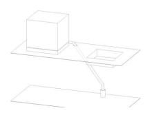
6. Fix drainage pipe on the sink with suction pad
