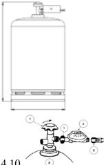
4.10 • Attach the pressure regulator to the gas bottle using the large brass nut. Always ensure that the rubber-sealing washer is present in the nut. (NB. This rubber washer is not required for UK-type pressure regulators). Tighten the nut and gas hose well. Note that the nut has a left-hand thread. Check the connections for leaks using a soap and water solution.
