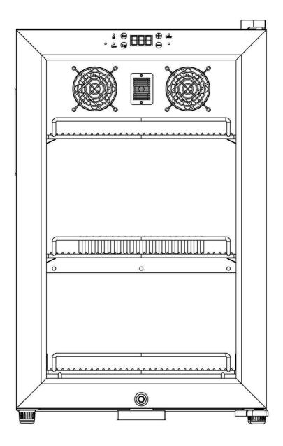
The temperature in the box can be adjusted from  $2^{\circ}$  C to  $8^{\circ}$  C
