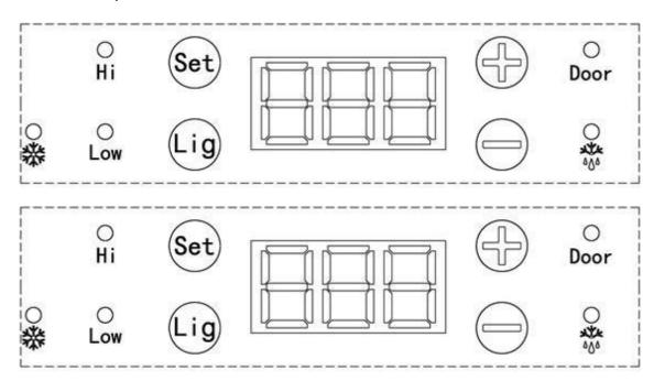
ON/OFF of the whole system ON/OFF of Inside Cabinet LED light
