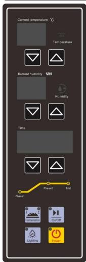
Fermentation setting: press button and its left light on, then adjust the time temperature and humidity by their buttons, then press "on/off" button to start working. If you need to set the second phase, you can press again and its
