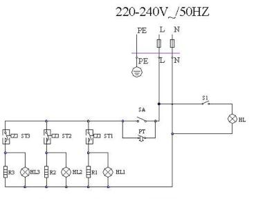
ST1 ST2 ST3 -Thermostat SA -Power Switch HL1 HL2 HL3-Indicator light S1-Switch of the internal lighting R1 R2 R3 -Heating element PT -Timer HL -Internal lighting
