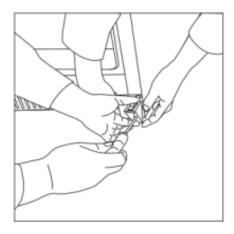
7.Tum the door up side down and connect to the upper hinge
