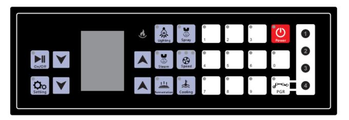
**Power switch**: long press 2s to turn on or turn off the power; short press once to reset (when you need to use other function, you can short press the power button, then choose the function you need).
