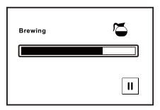
16 The pause button at the lower right corner allows you to pause the brewing processing case of emergency.
