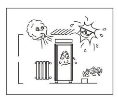
The cabinet must not be located in a chloride / acid-containing environment (swimming-bath etc.) due to risk of corrosion.
