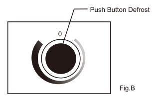
This refrigerator is equipped with a "push Button" (semi-automatic) defrost thermostat system. To activate the defrost cycle, simply push (in) the red defrost button located in the center of the control knob/dial. (do not turn the control knob/dial to zero=off). The defrost cycle is initiated immediately. When defrosting is complete, the "push Button" will release (pop-out) automatically and resume normal operating conditions at the same temperature setting.
